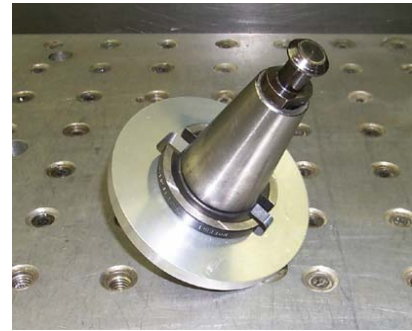
Fig 1.3 BT-40 tool holder with target disk mounted on it (Actual photo)
