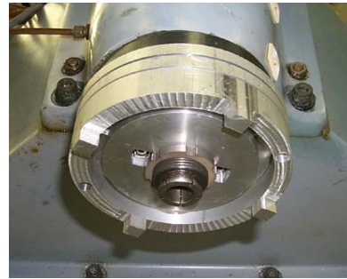
Fig 2.5 Mounts for the C1-B Capacitance gauges
