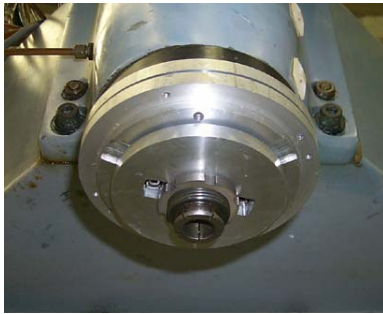
Fig 2.4 Target disk and tool holder
