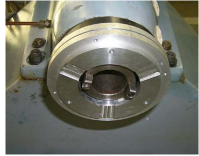
Fig 2.3 Mounts for the R1-A capacitance gauges
